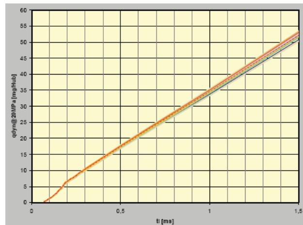
Fig. 8. Dynamic  $q_{\text{dyn}}$  characteristic
