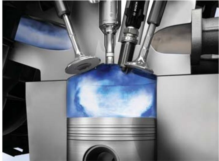
*Fig. 2. Jet-directed combustion system*
