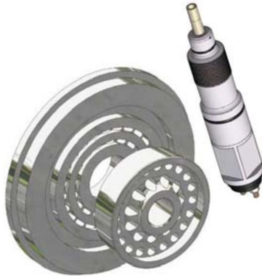
*Fig. 18. Solenoid actuated, outward opening multi ported valve plate injector for low pressure (early injection) DI operation of MAN urban transportation*
