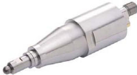
*Fig. 19. HyICE High pressure (late injection) DI: solenoid actuated needle injector; injector characteristics; flow area: 1 mm<sup>2</sup>, p<sub>cyl.max</sub>: 180 bar, p<sub>H2max</sub>: 250 bar*
