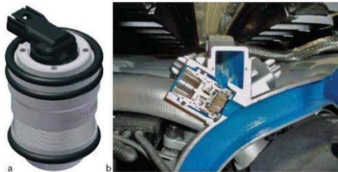
Fig. 16. Solenoid actuated inward opening ported valve plate injectors integrated into air manifold of BMW Hydrogen 7 car; injector characteristics: Flow area: 7 mm<sup>2</sup>,  $\Delta p_{max}$ : 5 bar.
