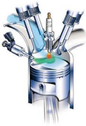
*Fig. 1. Wall-directed combustion system*
